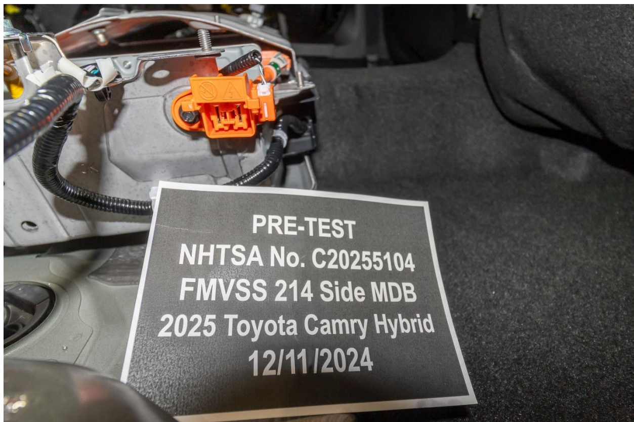
Figure 305-8: Manual High Voltage Service Disconnect Removed Location
