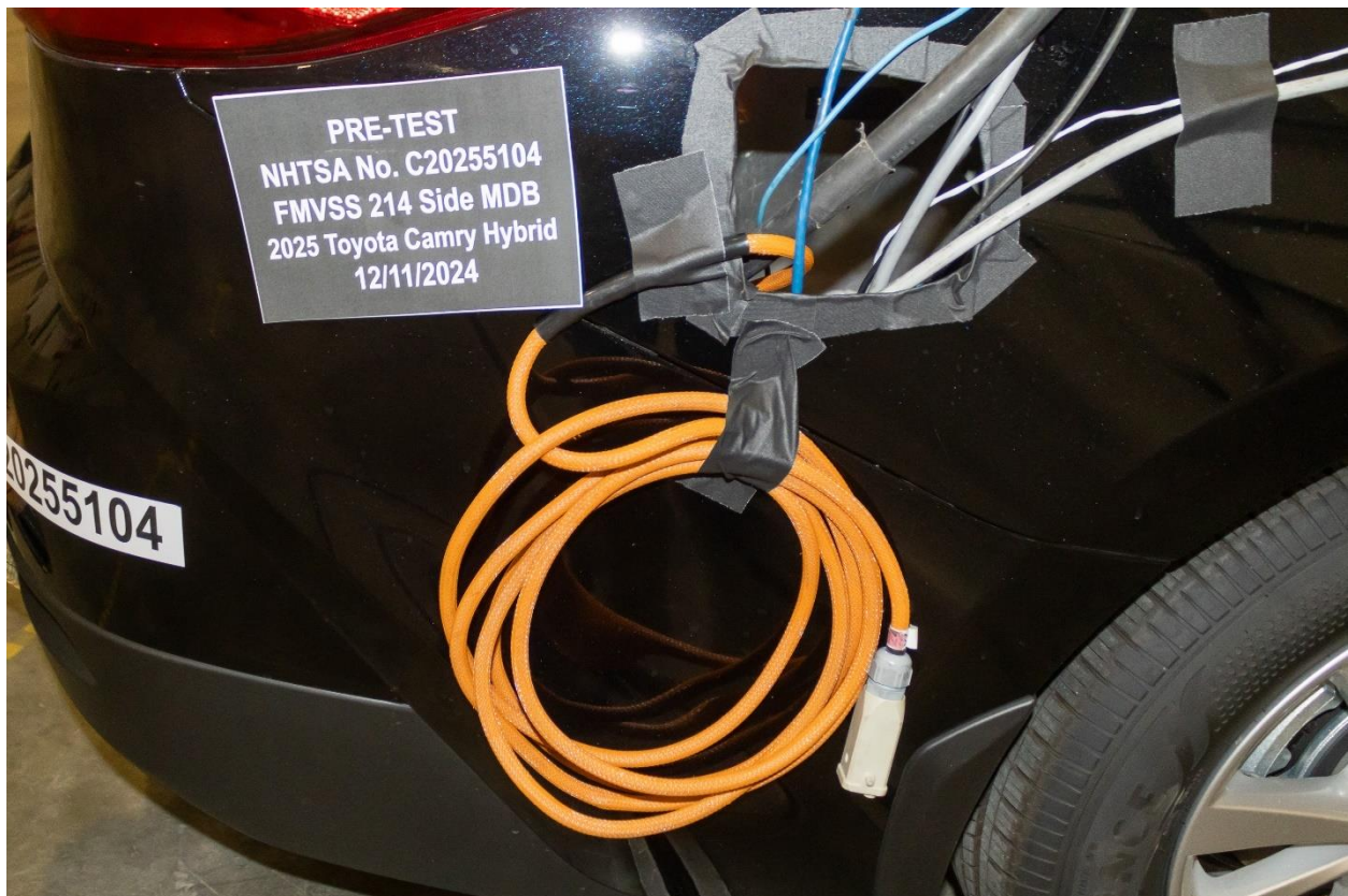
Figure 305-24: Pre-Impact View of Installed Test Interface Port
