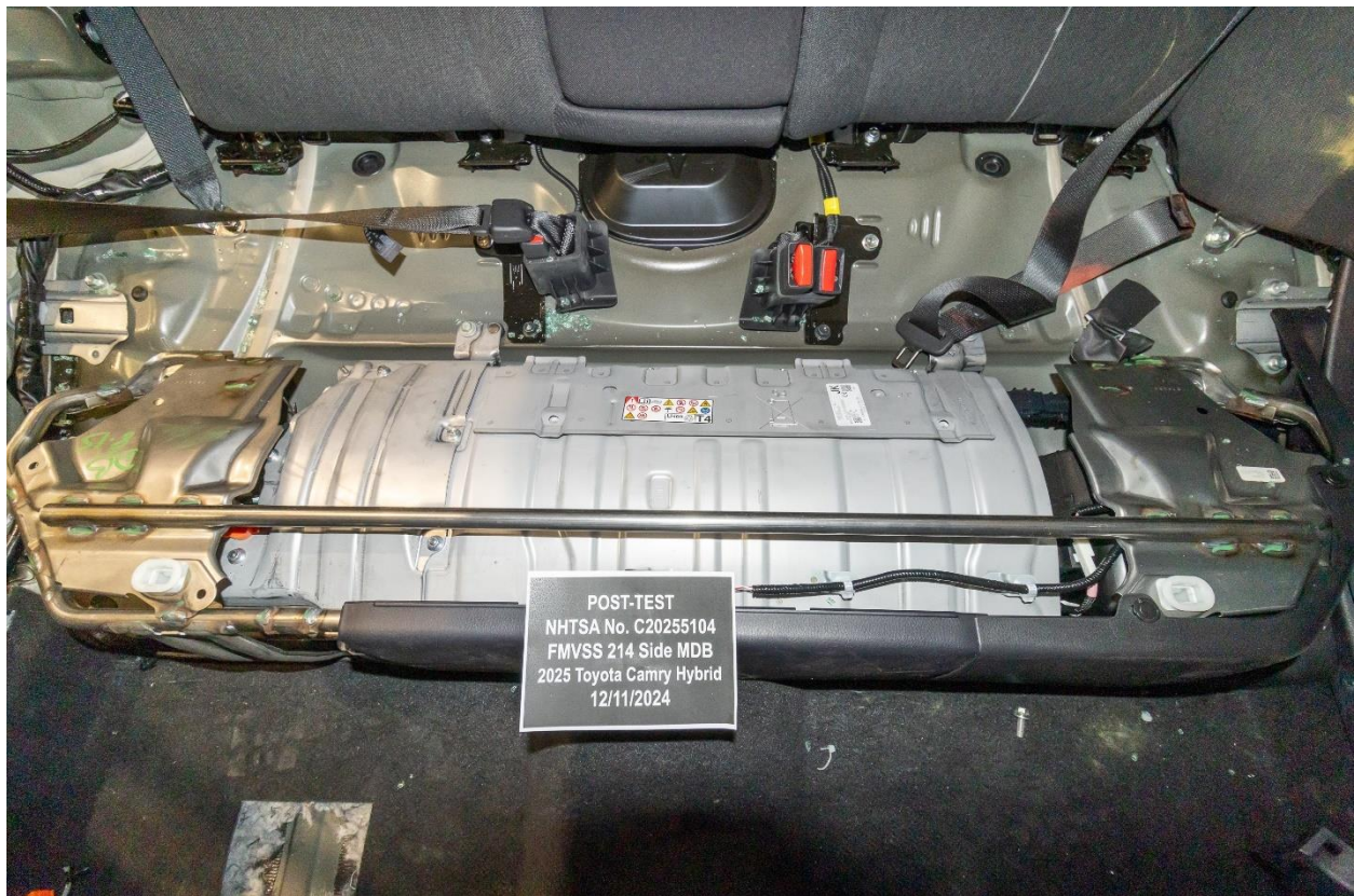
Figure 305-10: Post-Impact Front View of Propulsion Battery
