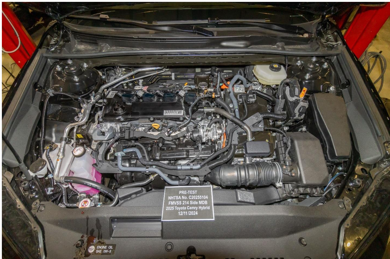
Figure 305-16: Pre-Impact View of Electric Propulsion Drive
